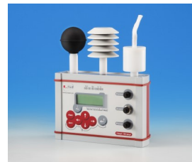
ELR600M / ELR610M: 5 cm diameter black globe sensor
