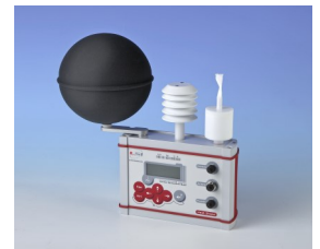
ELR605M / ELR615M: 15 cm diameter black globe sensor
