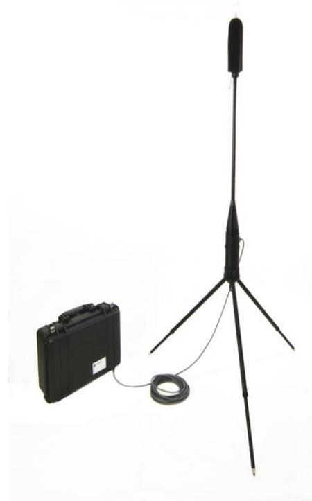
*\*The WK2 has a hook system at the top of the tripod legs to allow this to be chained down. The hook is on a standard 20mm conduit thread so that all the standard electrical fittings can be utilised to fasten the system in place. Some users mount the microphone on a vertical threaded conduit tube to place it at a special height\**
